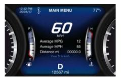
Further to speed, the main area can indicate three lines that can be set to the same options and in the top right or top left area. When these three lines are present and turn-by-turn navigation is on, main menu area will automatically show navigation information. For further details, please refer to MTC+ guide.
