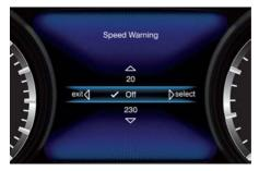
Scroll with the switch in the ▲ or ▼ arrow directions to view the selectable options.
