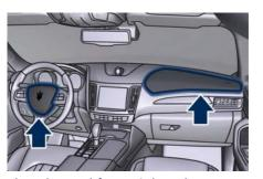
The advanced front air bags have a multistage inflator design. This allows the air bag to have different rates of inflation based on the severity and type of collision.
