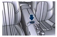
The storage and passenger compartment share the same air conditioning even though you may exclude the air conditioning of the cupholder compartment by moving the indicated button.
