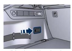
Pull the release cable moderately to avoid its possible break. It's not possible to feel or hear the unlocking of the fuel filler door actuator.
