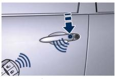
Press the lock button on the key fob RKE transmitter.
