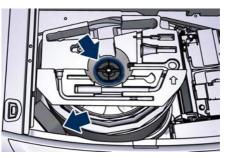
place the extension levers, the jack, the spanner and the adapter in the container inside the compact spare wheel;
