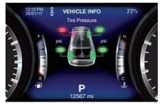
Should this occur, you should stop as soon as possible and inflate the tire/s with the low pressure (the one/s flashing in the instrument cluster graphic) to the recommended cold pressure inflation value. Once the system receives the updated tire pressure value, the system will
