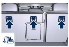
Such anchorages can be reached pushing down or lifting the foldable end of the trunk compartment cover.
