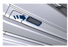
• remove the light from its seat and open the two parts to access the bulb:
