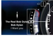
The system requires that the engine be running for all changes. When lowering the vehicle, all of the doors, including the liftgate, must be closed. If a door is opened at any time while the vehicle is lowering, the change will not be completed until the open door/s is/are closed.
