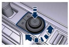
For further details, refer to "Infotainment System" in this section. When in App/Settings mode, the tune/scroll bottom knob and the browse ≡ and enter buttons allow you to scroll through the menus and change the user's settings (see "MTC+ Settings" in section "Dashboard Instruments and Controls").
