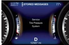
• Once you repair, replace or reinstall a tire with the compact spare tire, the TPMS will update automatically. The TPMS light (1) will turn OFF and the graphic in the instrument cluster will display a new pressure value instead of dashes (--), as long as no tire pressure is below the low-pressure warning limit in any of the four tires. The vehicle may need to be driven for up to 20 minutes above 15 mph (24 km/h) in order for the TPMS to acquire and process the updated information.
