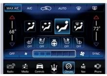
Front seats and steering wheel comfort setting soft-keys are present even when the A/C is off (see "Front Seats" and/or "Steering Wheel Adjustment" in section "Understanding the Vehicle" for further details).
