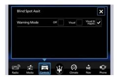
If the turn signal is then activated, and it corresponds to an alert present on that side of the vehicle, an audible chime will also be sounded: in the same moment the warning light will start flashing.
