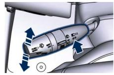
The left or right arrow on the speedometer and tachometer instrument cluster respectively, flashes to show proper operation of the front and rear turn signal lights.
