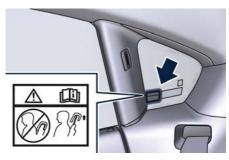
• To raise the head restraint, pull upward on the head restraint.
