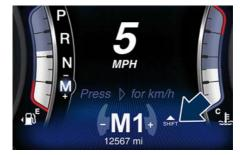
When the new gear is engaged, the indicator turns off. If the shift runs late or is not performed at all, the indicator remains lit for a few seconds then turns off. As soon as new conditions requiring further gear change occur, the indicator light will illuminate again.
