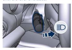
Flashing occurs also with lights off (lights switch in position "0") if the ignition switch is **RUN** position.
