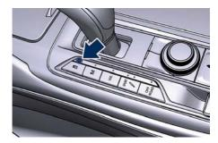
To deactivate the drive mode, press the same button again: the display will show the message indicating that \$\frac{1}{2}\$ (ESC OFF) drive mode is off and ESC system is active.
