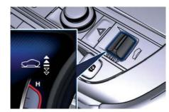
During transition from one position to another, the instrument cluster display will show a pop-up indicator (above the coolant temperature indicator) which reproduces the ride height symbols. On this indicator, the LED for the new position, set by means of the selector on central console, will flash while the LEDs of intermediate positions will turn on when set
