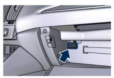
In the compartment of the central console there is also a SD memory card input. Once inserted into the slot, to extract it, press lightly on the card. For rear seat passengers, there are two USB ports inside the compartment located on the rear end of the central console, above the air vents. To access the USB ports open the outside cover.
