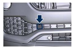
To access the rear tow hook seat, remove the external cap on the right side of the rear bumper.
