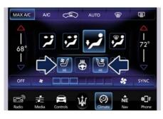
Within 15 seconds, touch the driver or passenger seat soft-key a second time to select LO-level ventilation.
