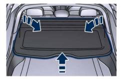
lift the cover rear end and slide it towards the liftgate: this will result in sliding the four lower ends of the cover inner part out of their guides on trunk panel;
