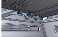
• remove trunk cover from the vehicle. The two parts of trunk cover can be folded one onto the other for a more compact unit.
