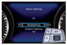
Use arrow ▲ or ▼ to scroll the list of parameters that can be adjusted and
