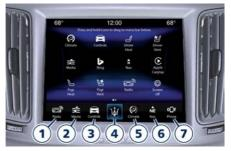
Main menu bar is set up by Maserati: it can be customized according to personal requirements, as explained in "Customizing the Main Menu Bar" in this chapter.
