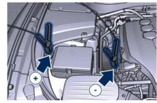
• Start the engine in the vehicle that has the booster battery, let the engine idle a few minutes, and then start the engine in the vehicle with the discharged battery. If using a portable battery booster, wait a few seconds after connecting the cables, before starting the booster vehicle.
