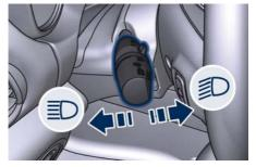
You can signal another vehicle with your headlights by lightly pulling the multifunction lever toward you. This will turn on the high beams headlights until the lever is released.
