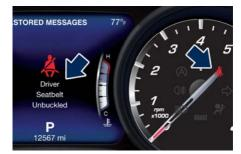
The BeltAlert® warning sequence begins after the vehicle speed is over 5 mph (8 km/h) for more than 19 seconds, by blinking the seat belt reminder light ¼ and message and by sounding an intermittent chime. Once the sequence starts, it will continue for the entire duration. After the sequence completes, the seat belt reminder light ¼ remains illuminated until the respective seat belts are fastened and the message remains on for 5 seconds.
