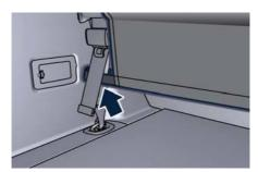
Should it be necessary to position the Cargo Net in position **B** - more forward, i.e., behind the front seats - use the top retainers next to external rear passenger handholds.
