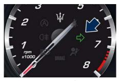
To activate lane change function, tap the lever up or down once, without moving beyond the detent. The turn signals (right or left) will flash three times then automatically turn off. This function is useful when overtaking or changing lanes.
