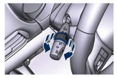
As a precaution, rear window washer pump stops if control is held in active position for over 20 seconds. When control is released, pump will resume normal operation.
