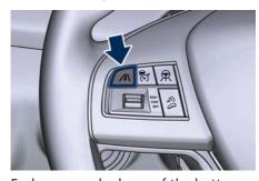
Each press and release of the button changes the gap starting from 3 bars (default distance) and moving in a sequential way towards the minimum distance:  $3 \rightarrow 2 \rightarrow 1 \rightarrow 4 \rightarrow 3 \rightarrow 2 \rightarrow 1 \rightarrow 4$  and so on.
