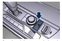
Press the switch to turn on the hazard warning flashers to warn oncoming traffic of an emergency. When these lights illuminate, the turn signals, the related indicator lights on the instrument cluster and the button start flashing.
