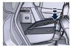
Now that seatbacks are folded down, trunk floor and the back panels of seatbacks will form a larger flat floor.
