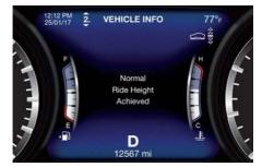
Driving vehicle before the set riding height is reached is not safe and could damage suspension components.
