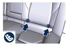
In addition, there are tether strap anchorages behind each rear seat.
