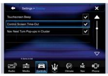
• Nav Next Turn Pop-ups in Cluster By selecting this feature, the next turn direction will appear on the instrument cluster along a programmed route until the desired destination is reached (see picture).
