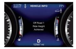
Set ride height and drive mode can be monitored on instrument cluster display via "Drive mode" menu, using buttons on the right-hand side of the steering wheel (see chapter "Instrument Cluster" in section "Dashboard Instruments and Controls").
