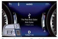
To turn the system off, push the ON/OFF button a second time or the ACC button (in the Optional Configuration). The No white light will turn off.
