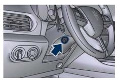
To lengthen or shorten the steering column/wheel, pull the switch toward you or push the switch away from you as desired.
