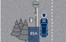
The BSA system will not alert you of objects that are traveling in the opposite direction of the vehicle in adjacent lanes.
