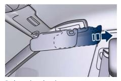
By lowering the visor you can access the courtesy mirror and, by sliding the mirror protective cover, the light on the dome will automatically light up (with the ignition switch in **RUN**). Before raising the visor, close the mirror cover: the light will turn off. A business card holder is fitted inside each sun visor.
