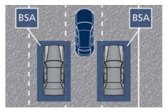
The BSA system monitors the detection zones on both sides of the vehicle when the vehicle speed reaches approximately 6 mph (10 km/h) or higher and will alert the driver of vehicles in these areas.
