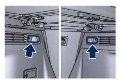
If liftgate is left open for a long time, lights will turn off after 30 minutes to save battery charge.
