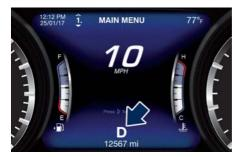
By pressing the release button on the lever, the gear position field is displayed: if you release the button without moving the lever, the field disappears after 2 seconds. By operating instead the lever, the new range will be indicated in the field and in the lower part of the display.
