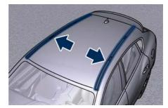
Weight of luggage/equipment carried on the rails must not exceed 176 lb (80 kg) and must be evenly distributed. This weight must be added to the load carried inside of the vehicle as well as the passengers' weight, and total must not exceed the maximum allowed weight (see "Features and Specifications" in section "Features and Specifications"). When arranging load on rails, make sure that it will not interfere with power liftgate and sunroof opening (if equipped).
