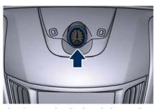
The time can be displayed also on the MTC+ main menu bar and on the instrument cluster display (see "MTC+ Settings" in this section). Clock lighting works in the same way as instrument and controls backlighting (refer to "Lights" in section "Understanding the Vehicle").
