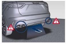
In order for the sensors to detect your foot movement, move your foot towards the vehicle rather than sideways and immediately pull it back: from this moment, the power liftgate will activate within two seconds. If closed, with the foot movement the power liftgate will:
