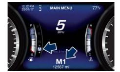
Using the shift paddles behind the steering wheel (if equipped), the corresponding icon will be displayed beside the "M" indication and current shifted gear.
