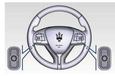
Press any button to display information on the radio station or track being listened to inside a pop-up for 2 seconds on instrument cluster. The right-hand control manages the volume.
