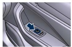
There are single window controls on each passenger door trim panel, which operate the corresponding window. The window controls will operate only when the ignition switch is in the ACC or RUN position.
