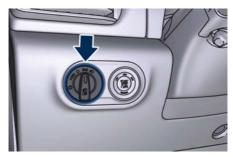
Rotate the light switch to the or to the position: the instrument cluster will display the related telltale.
