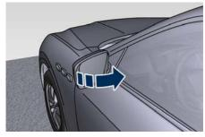
Press the switch once and the mirrors will fold in; press the switch a second time to reset the mirrors to the standard position.
