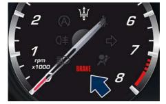
During engagement and disengagement procedures, the warning light **BRAKE** flashes until the parking brake has reached its maximum activation force and is respectively fully released. In the above-mentioned conditions, the automatic engagement function can be deactivated/activated by selecting the menu item "Vehicle settings" on the main menu (refer to paragraph "Deactivating Automatic Operation" in this chapter).
