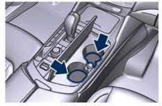
By pressing the indicated button on the central console, the half-lids will rise completely enabling access to the inner compartment where the two cupholders are located.
