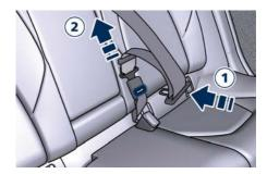
Allow the belt to retract completely into the retractor seat behind the seatback.
