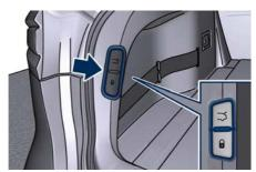
Each time the vehicle security alarm is armed, the anti-intrusion and anti-lift sensors actively monitor the vehicle. When arming the security alarm, it is possible to disable these sensors by pressing the button on the key fob three times within 5 seconds from the moment the system has been armed (meanwhile the security alarm light flashes rapidly).
