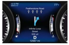
While getting closer to a turn, the sections referred to the distance already traveled will switch off while the ones referred to the distance yet to be traveled will remain on.
