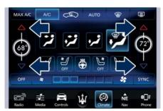
To provide you with maximum comfort in the Automatic mode, during cold start-ups the blower speed will remain low until the engine warms up.
