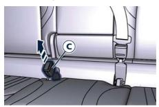
Insert the latch plate located at the end of the lap portion of the belt (A) inside the right buckle (C).
