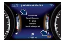
Initialize the EPB System after Re-connecting the Vehicle Battery After the detachment and the subsequent connection of the battery, on the instrument cluster display the warning light (P)! will be illuminated. To initialize the EPB system, lift, release and lift again the lever located behind the shift lever.
