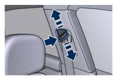
When you release the anchorage try to move the belt slider up and down to make sure that it is locked in position.
