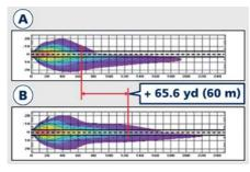
Combining a bending mode and a vertical adjustment, the system assures better visibility of the road surface when driving on a curve, steering, or in the event of road deviations, optimizing vertical and horizontal light distribution according to the current drive path.
