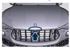
Slightly lift the hood and push the safety catch as indicated by the arrow. The safety catch is located in the center of the hood.
