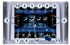
To adjust driver and passenger side temperature and fan speed, climate control panel features two-function controls that can be pushed up to increase temperature/speed, or down to decrease them.
