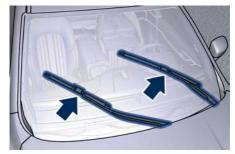
It is possible to use the "MIST" position for a maximum of 3 times within two minutes, corresponding to different three blades positions on the windshield. When completed, bring the ignition switch in **RUN**: the arms will reposition. If necessary move the multifunction lever to other required operating positions.
