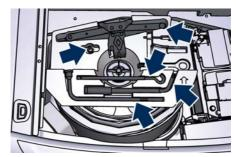
• Unscrew and pull out the locking wheel knob.
