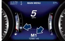
In normal conditions, the shift lever is always unlocked. When in D (Drive) mode it is possible to upshift or downshift the changing gears by automatically temporarily setting in M (Manual) mode.
