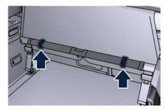
Attach the lower side ends of the Cargo Net to the tethers, using the Velcro appendices indicated in the figure.
