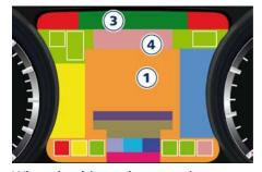
When the driver selects a main menu page and the Traffic Sign Assist (TSA) feature on "Controls" page of MTC+ is set off (see "MTC+ "Controls" Screen" in this section), main menu title, its number and the scroll arrows will disappear after two seconds. When driver selects a main menu, if the TSA feature is set on and a sign and/or a speed limit icon is displayed in sector 23, only the main menu number and the scroll arrows remain displayed in the sector 3, left side.
