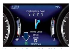
The amber indicator light **Q**≢ inside the tachometer of the instrument cluster illuminates when the rear fog lights are turned on.
