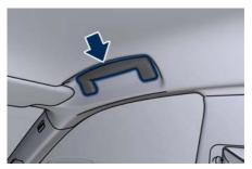
Behind the rear handholds there is a light with relevant on/off switch (refer to chapter "Lights" in this section). Cloth hooks are present on rear handholds and on pillars between doors.
