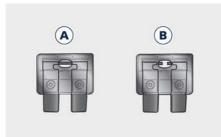
The vehicle mainly uses mini-and maxi-fuses with blade engagement. Besides these there are other types of fuses provided with holes for attaching to the cable connection terminals.
