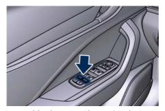
To enable the controls previously described, press the window lockout button again (setting it in the up position).
