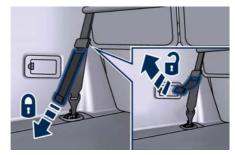
• Freeing the net lower part from the Cargo Net structure.
