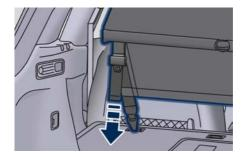
When Cargo Net is no longer necessary, release the net lower part
