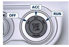
In case the ignition switch does not change by pushing a button, the RKE transmitter (key fob) may have a low or discharged battery. If this occurs it is necessary to replace the battery in order to operate the ignition switch (see "Requiring and Setting Additional Key fobs" in this section).
