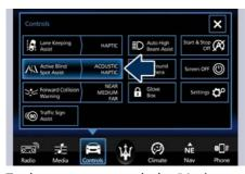
To change status, touch the "Active Blind Spot Assist" soft-key. To change the system setting, touch the soft-key on the side.
