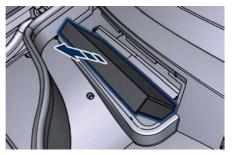
Install the new filter with arrows pointing in the direction of airflow, which is toward the rear of the vehicle (text and arrows on the filter will indicate this).
