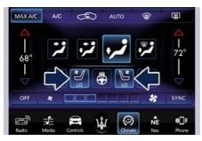
Within 15 seconds, touch the same soft-key a third time to shut off the seat ventilation.
