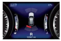
As the vehicle moves closer to the object, the instrument cluster will display the arc moving towards the vehicle and the sound tone will change from single to slow, to fast and to continuous.
