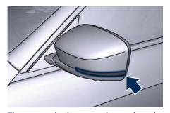
The external mirrors can be equipped also with approach and courtesy LEDs, lighting up when the vehicle entry/exit lights are activated.
