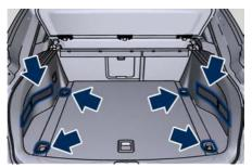
Longitudinal rails on trunk floor provide safe anchorage for luggage of different size, thanks to the special hooks with locking button. To position the hook, slide it along the rails until reaching the required position, holding down the central button. Release the button and slightly move the hook to secure its position in the notches of the guide.
