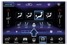
Within 15 seconds, touch the heated steering wheel soft-key to turn on the function.
