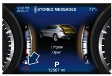
With the ignition device in the OFF position, only the power liftgate open symbol will display until closure. See "Passive Entry System" in this section for more information on power liftgate operation with the "Passive Entry" feature.
