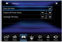
• Engine Off Power Delay (Power duration after engine shutdown) By selecting this feature, the power window switches, radio, MTC+ Phone System, power sunroof (if equipped), and power outlets will remain active for up to 10 minutes after turning off the engine.
