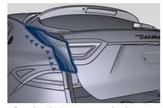
After the closing command, when power liftgate starts closing, all the indicators will blink to warn anyone within range.
