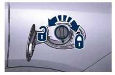
• When refueling, place the cap in the proper seat on the filler door hinge.
