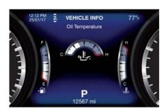
The gauge fill and telltale (if applicable) are highlighted in red to emphasize that the parameter is at a critical level.
