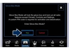
Unlock glove box by entering the lock code as previously specified.
