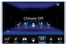
When the MTC+ System is in any mode other than "Climate" ("Radio", "Media", "Controls", etc.) the driver and passenger temperature settings will be indicated on the upper part of the display.
