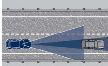
HAS combines ACC and LKA to manage the steering and speed of the vehicle under specific conditions. The conditions to engage HAS are listed in the next paragraph. If a lane line cross is imminent, the steering wheel will
