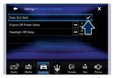
Once the procedure is completed (for example, Display mode) touch the ← back arrow soft-key to return to the previous menu or touch the upper right "X" soft-key, to close the settings screen. Touching the ▲ or ▼ soft keys and the cursor on the right side of the screen will allow you to scroll up or down through the available settings.
