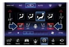
Within 15 seconds, touch the same soft-key a third time to shut off the seat heating.
