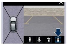
In the top view, the vehicle is represented as it is during the maneuver (see example in the figure), therefore any open doors will be visible in the image.
