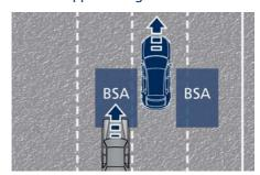
When the vehicle is started, the BSA warning light will momentarily illuminate in both outside rear view mirrors to let the driver know that the system is operational and on. The BSA system sensors operate when the
