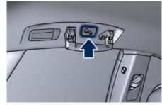
Lower the handhold and engage the net top ends in the slot on roof, as already described for the rear retainers.
