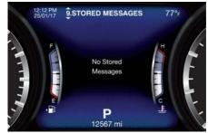
Press and release the switch in the ▲ or ▼ arrow directions to scroll the stored messages.
