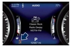
This warning light informs the driver that FCW is disabled. This warning light will light even when the activation of another driver assistance feature or drive mode (example: (ESC OFF)) disables the FCW.
