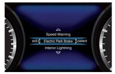
Press and release the switch once again toward the arrow ( ▶ ) to visualize the options connected to this function.
