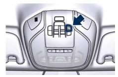
After pressing the button the instrument cluster will display the state of front parking sensors for approximately five seconds. The button LED will be on when the front sensors are disabled. The button LED will be off when the front sensors are enabled. If the button is pressed and
