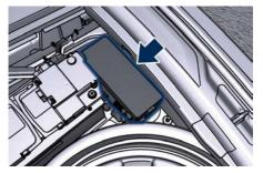
on the fuse and relay box located in a covered area, under the dashboard left side.
