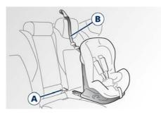
LATCH-Compatible child restraint systems are now available. You should never install LATCH child seats so that two seats share a common lower anchorage.
