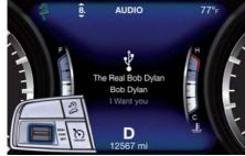
Push up (RES +) multifunction switch to increase speed until the required value is displayed below the green light on display.
