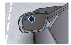
The external of the rear-view mirror support is equipped with LEDs, lighting up when the turn signals and vehicle entry/exit lights are activated. When the surround view camera system is installed, at the external bottom side of the rear-view mirror is the side view camera (refer to "Surround View Camera System (optional)" in section "Before Starting").
